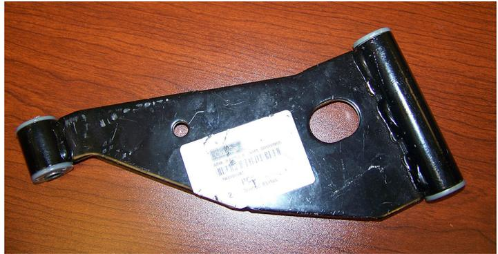
To install the new bushings clean the bore and clean off any burrs that may exist.
